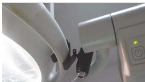
In OT, Wi-Fi enabled camera fixed to OT light for allowing operating surgeon to interact with other surgeon (Tele-OT Consultation)
